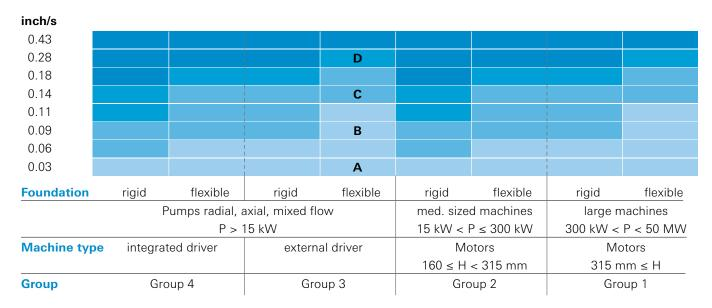
**DIN ISO 10816:** Mechanical vibrations – assessment of the vibrations of machine through measurements on no rotating parts. **Vibration velocity (rms)**  $10 - 1000 \, \text{Hz}$ ,  $n > 600 \, \text{min}^{-1}$ ,  $2 - 1000 \, \text{Hz}$ ,  $n > 120 \, \text{min}^{-1}$
